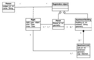
Figure 8. Proposed Class Diagram to register Apartment Unit (Suhattanto,2009:72)
