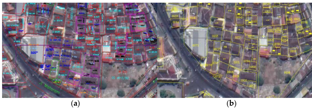
Figure 3. (a) Working map (the initial product of the mapping process); (b) GeoKKP parcel map (map of the final results of the plot mapping process, stored in the GeoKKP database on the central server).
